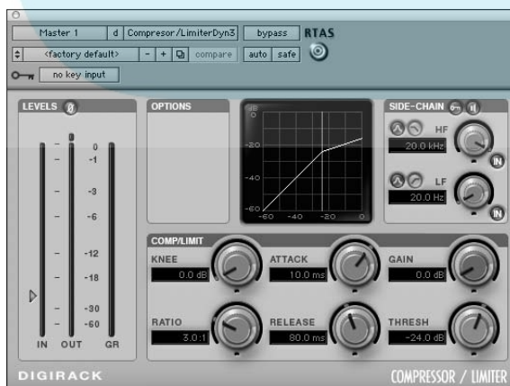
Figure 4-2: Use the Pro Tools Compressor/Limiter plug-in to adjust several parameters to even out your sound.
